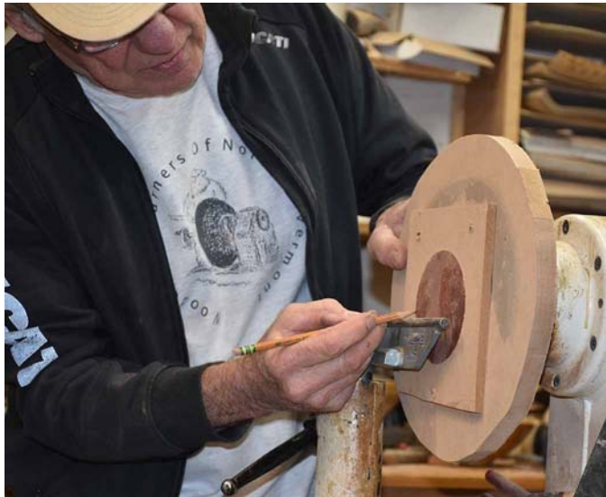
Russ draws a pencil circle as a starting point for the cuts.
