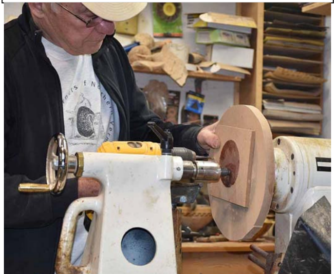
A pre-cut round is pressure-fitted into an MDF square. Russ prefers to cut into the off-set side of the workpiece first. Here, he mounts the square onto a round of MDF mounted on the lathe.
