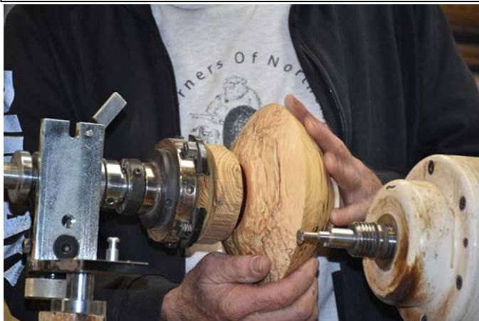
The lid having been threaded, Russ fits the box onto it. This version of the Hope tool has a hinge for easy working and trial.
