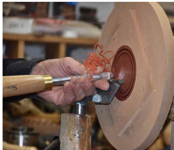
Circles are cut, centered on the piece and just deep enough to impinge on the circles cut on the other side of the workpiece.
