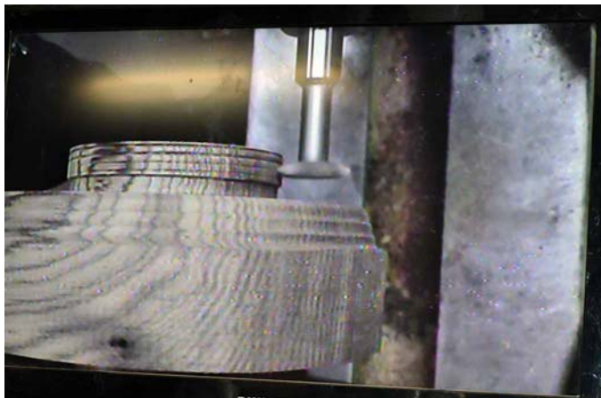
The Hope thread cutter rotates and advances the workpiece.
