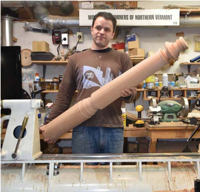
Nick got a commission to do some BIG spindles! He did about 5 near-identical Newell posts using a cardboard template.
