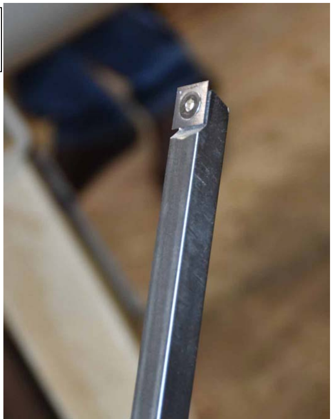
Ted Latrell made some carbide-tipped tools using available steel stock and cutters.
