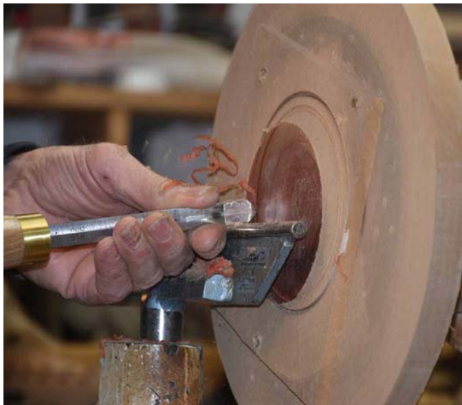
The outside circle is being cut. The square of MDF keeps the workpiece from splintering at the edges.
