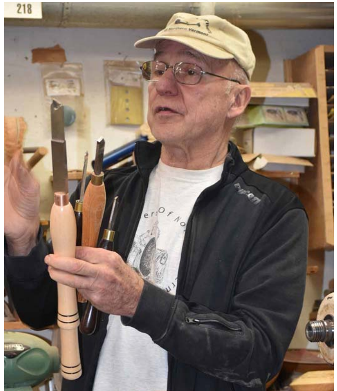
Russ uses several parting tools to produce his concentric cuts.
