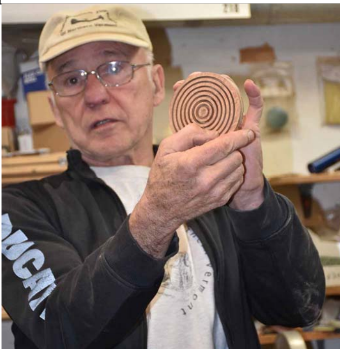
The cuts need to be evenly spaced and evenly deep.
