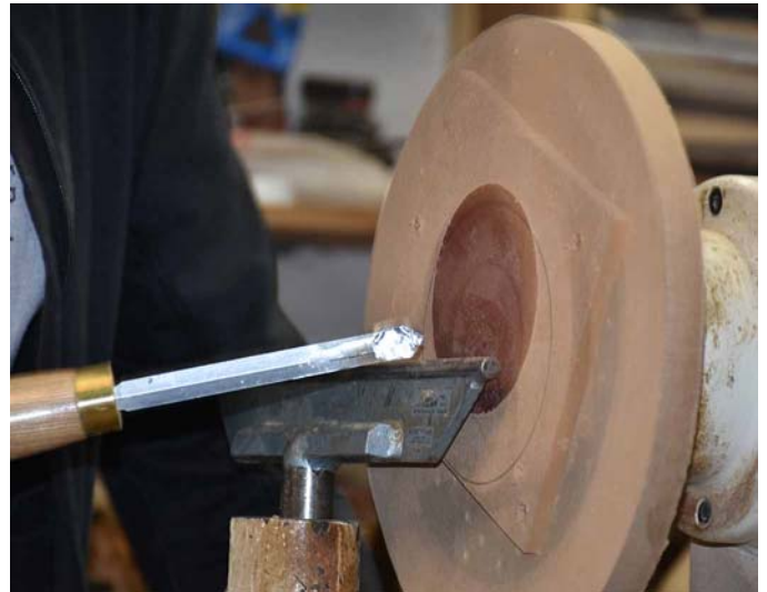
This parting tool has aluminum tape to mark the cut depth.
