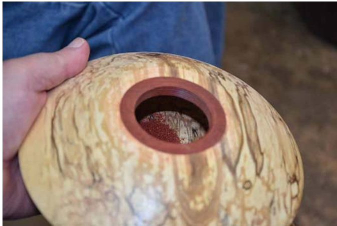
Russ installed a piece of even-grained hardwood as the spalted wood could not take thread-cutting.
