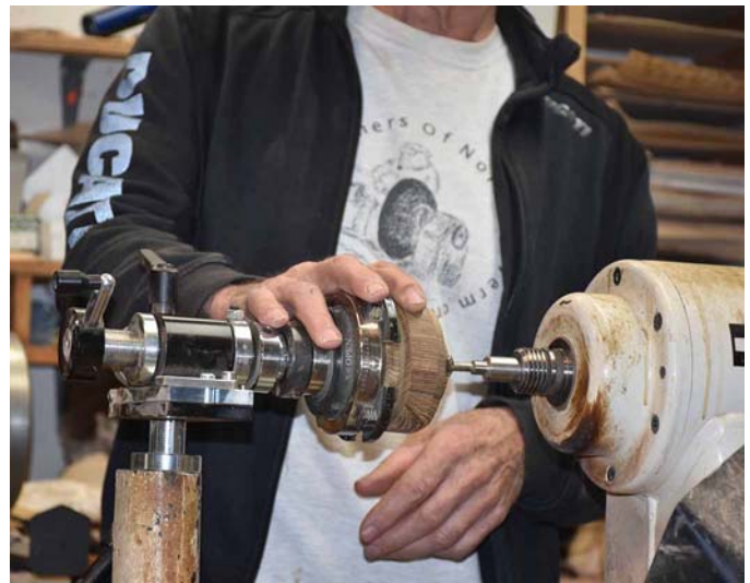
Russ mounts a workpiece on his lathe. The cutter is driven at high speed. The workpiece is rotated in the chuck jaws against the cutter.
