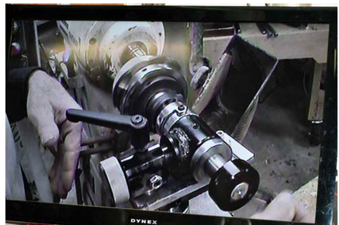
Russ advances the tool one click at a time to deepen the cut.
