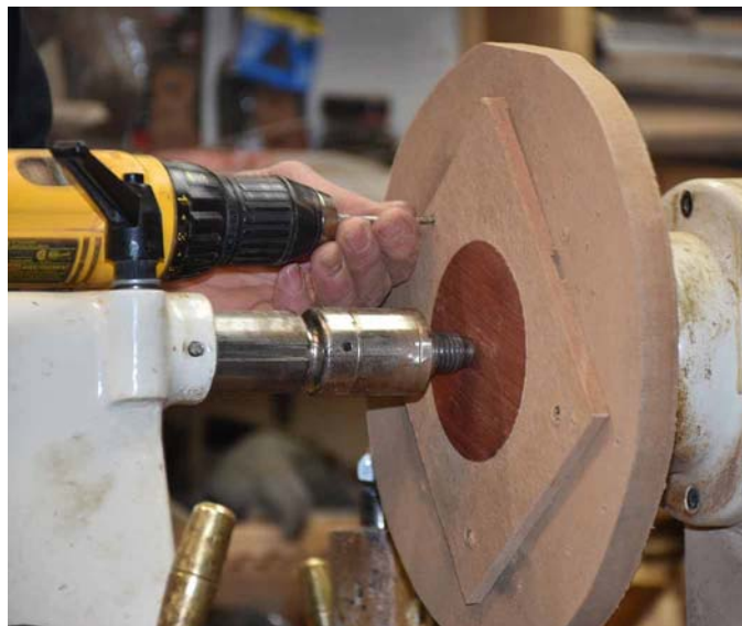
The piece is flipped and fastened centered to the MDF
